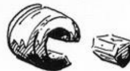
Repaired Rear Wing Mount using.....section of rear tyre
